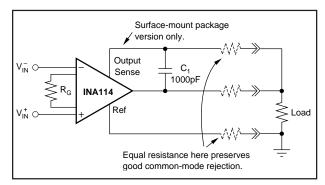
FIGURE 5. Remote Load and Ground Sensing.
