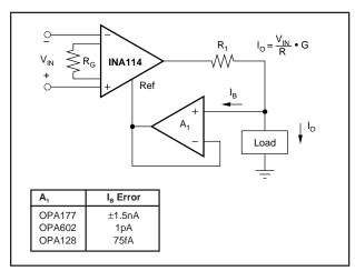
FIGURE 13. Differential Voltage-to-Current Converter.
