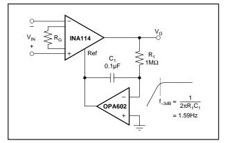
FIGURE 12. AC-Coupled Instrumentation Amplifier.
