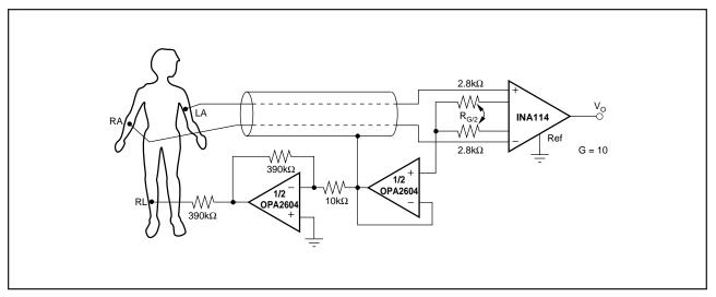
FIGURE 10. ECG Amplifier With Right-Leg Drive.
