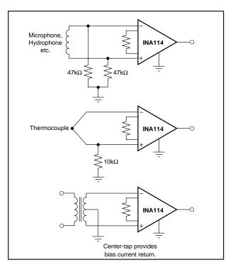
FIGURE 3. Providing an Input Common-Mode Current Path.
