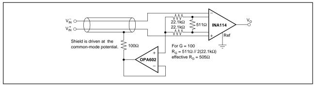
FIGURE 7. Shield Driver Circuit.
