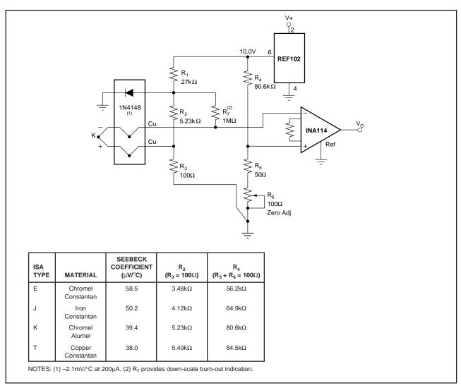
FIGURE 9. Thermocouple Amplifier With Cold Junction Compensation.
