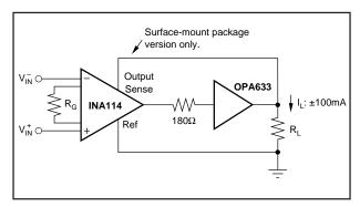
FIGURE 6. Buffered Output for Heavy Loads.
