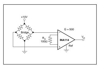
FIGURE 11. Bridge Transducer Amplifier.
