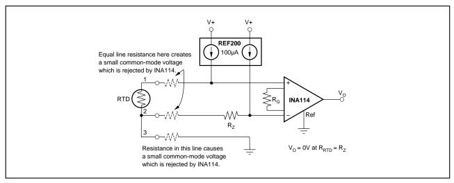
FIGURE 8. RTD Temperature Measurement Circuit.
